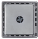
0306-10-79S1 Floor Drain SUS 304 Size 125*125 mm Height 65 mm Seal Type Self Seal ABS Flow Rate \geq 18 L/Min Outlet OD 42.0 mm Drain Core 0305-A1-7900
