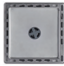
0306-12-79S1 Floor Drain SUS 304 Size 102*102 mm Height 65 mm Seal Type Self Seal ABS Flow Rate \geq 18 L/Min Outlet OD 42.0mm Drain Core 0305-A1-7900
