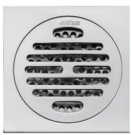
0303-62-79CP Floor Drain Brass Size 100*100 mm Height 43 mm Seal Type Self Seal Brass Flow Rate \geq 15L/Min Outlet OD 40 mm Drain Core 0303-A1-7900
