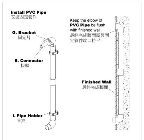
\* Use **Bracket** and **Pipe Holder** to help to fix and install the **PVC Pipe**, and please make sure to keep the elbow of **PVC Pipe** be flush with finished wall.
