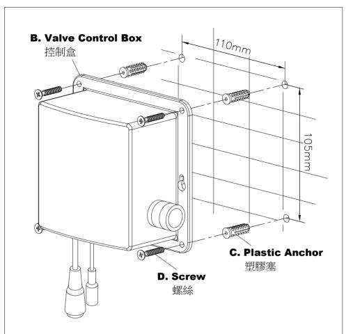
\* 1. Select proper position to install the **Valve Control Box** (It's better to be lower than plug), use box to mark the positions of drilling holes.
