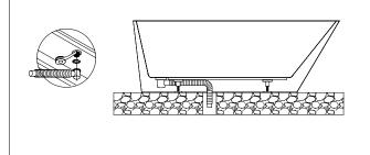
4. Finally you need to do a fnal test for drainage. Ensure that the thin masking plastic adhered to your bath during manufacture has been removed . Fill the Bath with water and check that ALL the water flows freely to the waste
