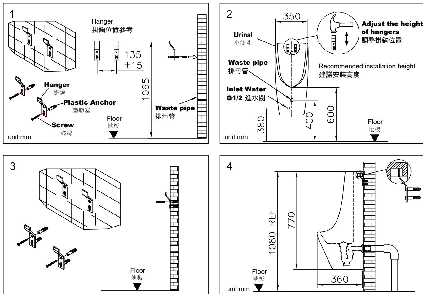
**⚠ Please carefully confirm the installation instructions of the electromagnetic valve and urinal before installation.**
