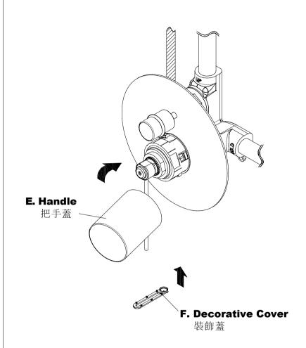
\* Insert the lever through a hole in the **Handle**. Then fix the **Handle** and the **Decorative Cover**.
