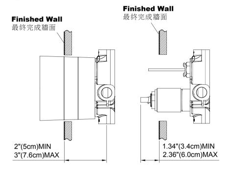
\* Connect hot and cold supply pipes to the valve body and meantime install outlet water ways, and keep the distance between 2"(5cm) minimum and 3"(7.6cm) maximum from the finished wall to the valve body; or keep the distance be 1.34"(3.4cm) to 2.36"(6.0cm) between top of cartridge and **Finished Wall** for necessary conditions.
