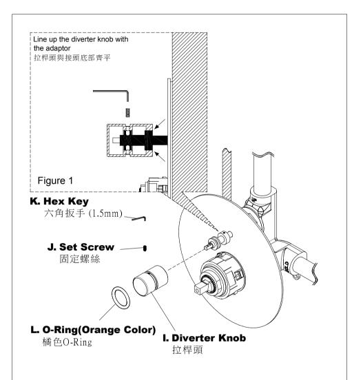
\* Slide the **Diverter Knob** onto the **Adaptor**. Line up the **Diverter Knob** with the **Adaptor** as shown on the figure 1. Use the **Set Screw** to secure knob's position. Put the **O-Ring** on the knob's body.
