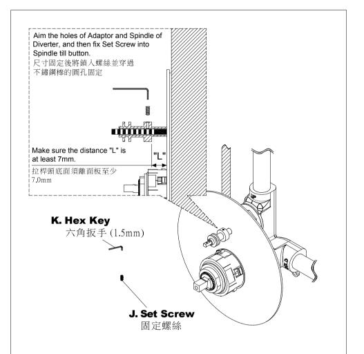
\* Make sure the distance "L" is at least 7mm. Adjust **Adaptor** to proper position, aim the holes of **Adaptor** and **Spindle of Diverter**, and then fix **Set Screw** into Spindle till button.
