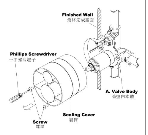
\* Carefully remove the **Sealing Cover** by removing two **Screws**.
