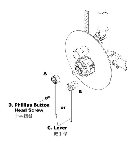
\* Select the right **Lever**. Slide the lever onto the cartridges stem. Tighten it with the **Screw**. P.15 will explain how to select the right **Lever**.
