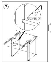
Make sure the two pillars are vertical to the floor, then complete tighten the Connection-Pipe by 3mm Hexagon Key.
