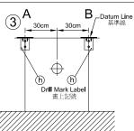
Place each of the **Drilling Templates** right beneath the intersection of datum line and line A (& B).
