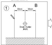
Mark two lines A & B both sides 30cm(12") from the center of drain outlet .
