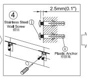
Using A NO.16(8mm) bit, drill screw holes in the position marked to A depth of 51mm(2") and insert Plastic Anchor flush with wall. Do not completely tighten Stainless Steel
