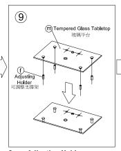
Screw Adjusting Holders on Tempered Plate Glass.
