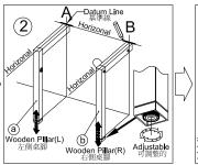
Level Wooden Pillars against the wall to A & B lines, adjust both
