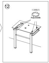
Level **Tempered Plate Glass** by twisting Adjusting Holders.
