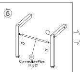
Join Connection-Pipe with Wooden Pillars; remain adjustable for the time being.
