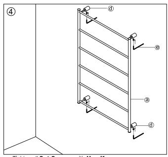
Tighten all Set Screws with Hex-Key. 用六角板手將所有埋頭螺絲鎖緊.
