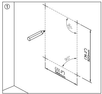
Mark 4 drill hole locations with a pencil on appropriate height position as shown in figure #1. 如圖1所示,在適當的高度用鉛筆在四個鑽孔的位置作記號.
