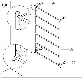
Twist pillars square to the wall and insert them into the **Brackets** as shown in figure #3. 如圖3所示,將柱子轉成與牆面垂直並且裝入支架.
