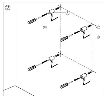
Lossen the Set Screw with Hex-Key then Drill fixing holes and installs 4 Brackets in positions.
