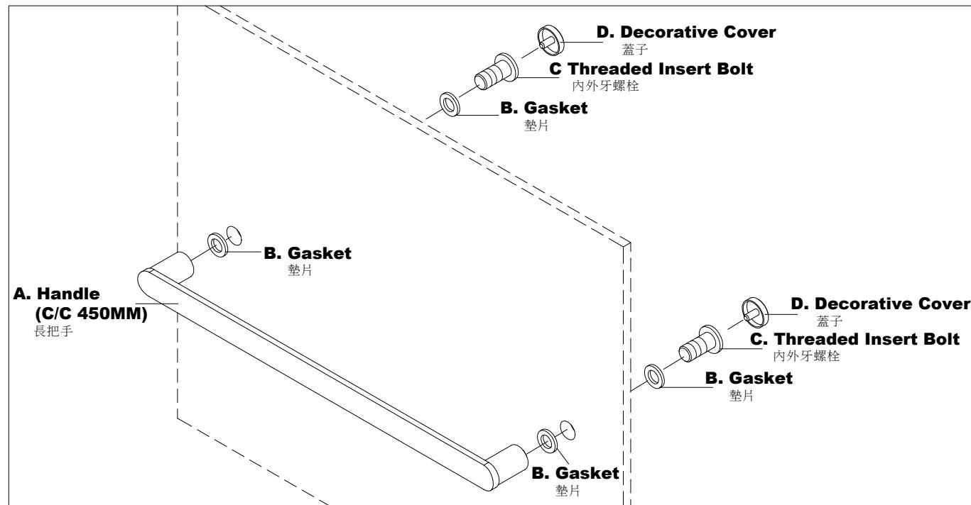
△ NOTICE 1. Available size of mounting holes is O/D15mm; available thickness of glass door is 8~20mm.
