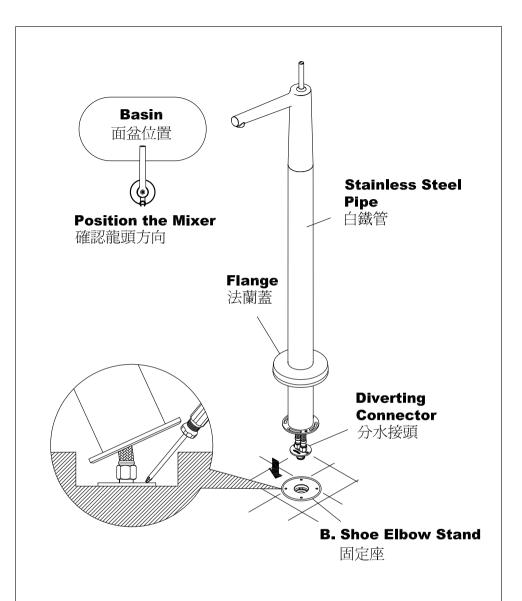
\* Position the **Basin Mixer** to Basin before installation, and press the **Diverting Connector** into the **Shoe Elbow Stand** with fingers and tools.
