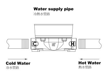
\* Connect the hot and cold water supply as the marks on the **Shoe Elbow Stand**. After finish the installation, please make sure if the connection of hot and cold water supply are same as the marked indication on the **Shoe Elbow Stand**.
