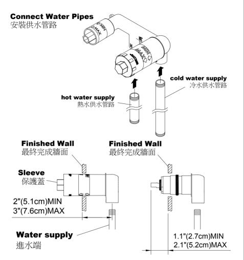
\* Connect hot and cold supplies pipes to the valve body, keep the distance between 2"(5.1cm) minimum and 3"(7.6cm) maximum from the finished wall; or keep the distance from 1.1" (2.7cm) to 2.1" (5.2cm) between top of cartridge and **Finished Wall** for necessary conditions.
