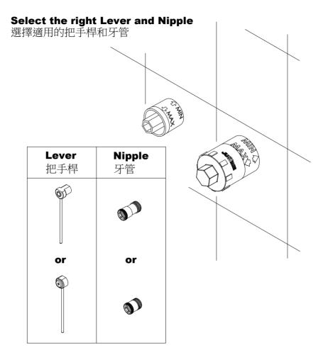
\* Before installing spout and handle, choose the proper **Lever** and **Nipple** according to the distance from top of the **Sleeve** to the finished wall.
