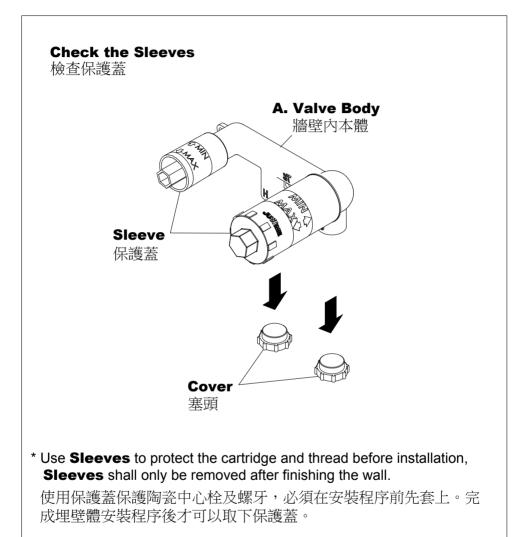
\* Remove the **Covers** of cold and hot inlets before installation. 安裝前請先移除冷熱水進水口塞頭。
