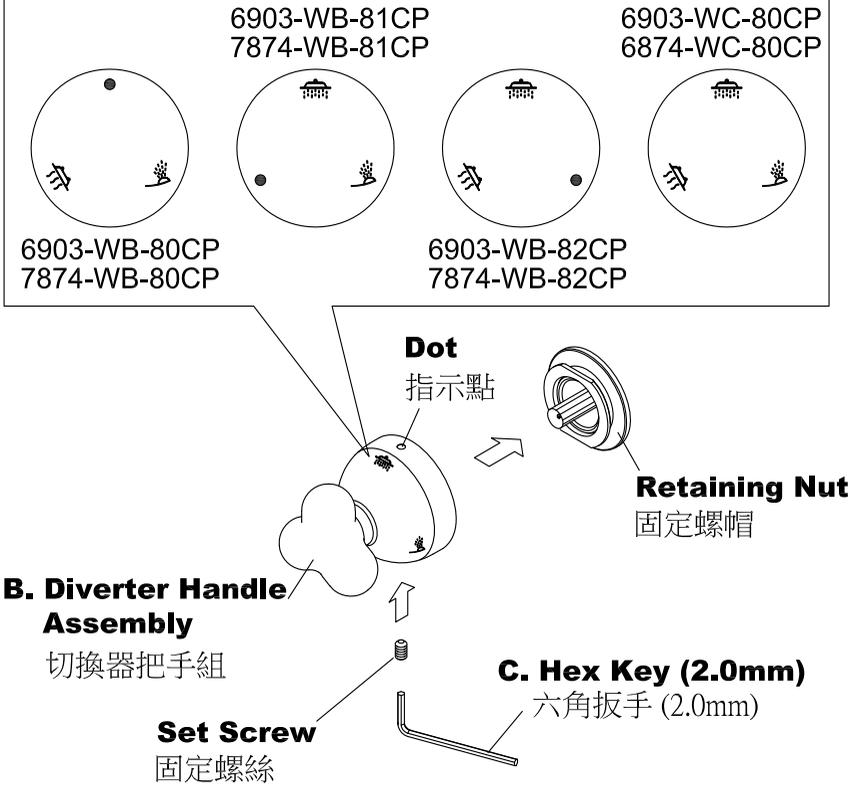
\* Align the **Rain Shower Sign** with **Dot**, and keep them be upward before installing. Fix the **Diverter Handle Assembly** onto the **Retaining Nut** by provided **Hex Key (2.0 mm)** and **Set Screw**.
