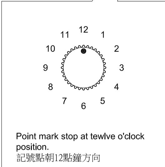
\* Face to the **Diverter Spindle**, and then adjust the **point mark** of **Diverter Spindle** to the twelve o'clock position.
