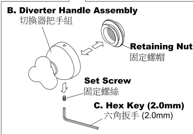
\* Disassemble the **Retaining Nut** from **Diverter Handle Assembly** with **Hex Key (2.0mm)**, and then fix the **Retaining Nut** to **Threaded Shank** until against finished wall.
